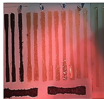
Figure 5. Tensile samples with different fiber weight ratio of Kevlar and Carbon fiber
