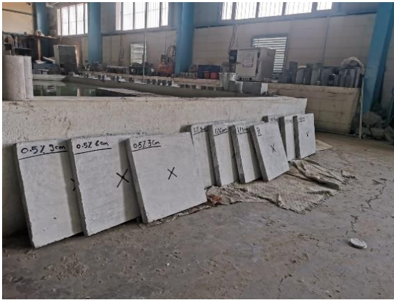
Figure 2. Concrete slabs (500 × 500 × 50) mm
