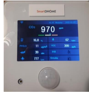
Figure 6. Sensor 9 in 1 including CO 2 concentration and motion (PIR) sensor used in the experiments ( https://www.smartdhome.com )
