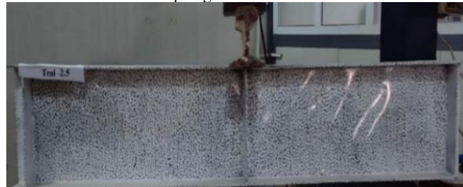
Triangle corrugated girder with a/d=2.5
