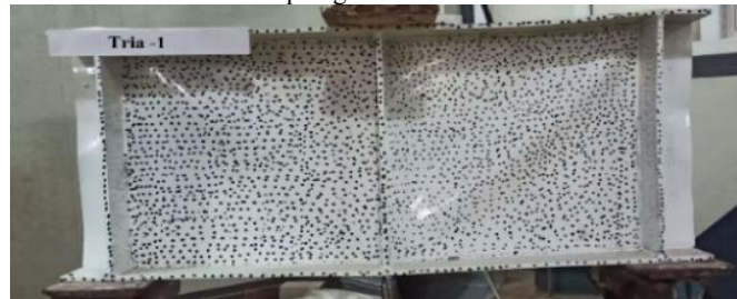
Triangle corrugated girder with a/d=1
