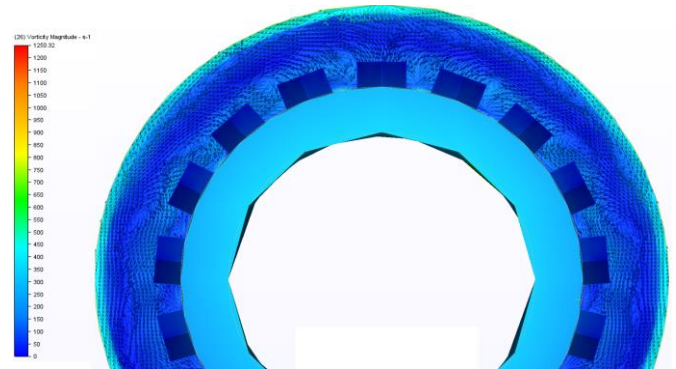
(a) Vorticity magnitude and velocity vectors behind VGs in annular space. Plane 6 from the left to right on (6c)
