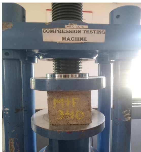
Figure 2. Compressive strength test
