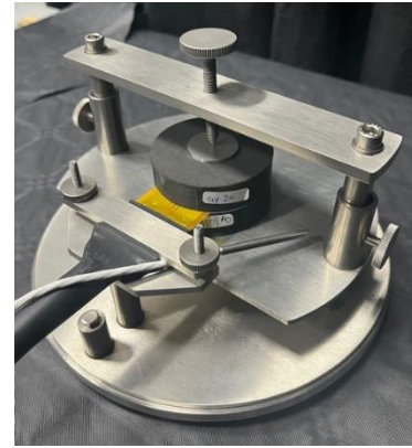
Figure 1. The sample set in the TPS 1000 without the steel cover
