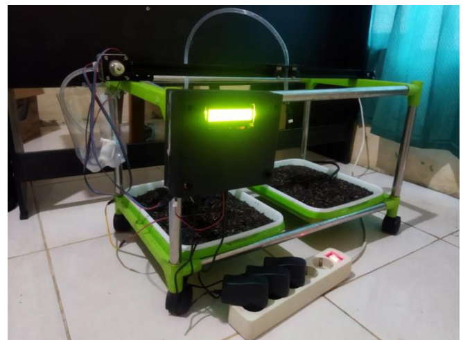
Figure 4. Prototype of automatic moving irrigation system
