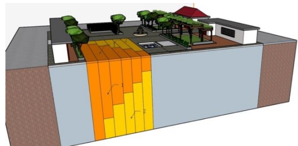
Figure 5. Watertight system Source: Study [86]
