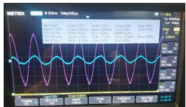
Figure 22. Grid-connected inverter voltage at the LCL filter output synchronized with grid voltage
