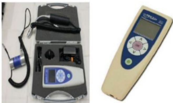
Figure 2. Airborne ultrasonic test equipment visualization [29]
