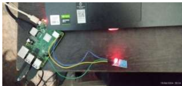
Figure 9. The suggested coldchain solution's designed sensing node
