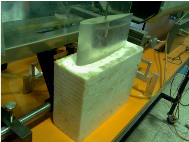
Figure 4. Model and cast which are fabricated to form an icy-airfoil
