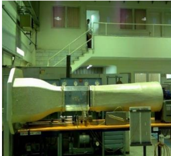
Figure 1. Subsonic wind tunnel which is used to measure the drag force on solid bodies
