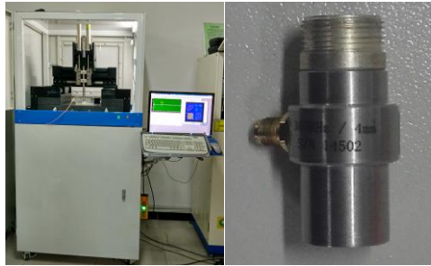
Figure 5. High-frequency scanning acoustic microscopy measurement system and high-frequency ultrasonic transducer
