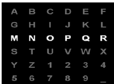
Figure 5. A matrix of alphabetical letters and other symbols is flashed in a random sequence in the BCI application [5]
