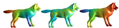
Figure 6. Real-valued functions visualized on wolf shape from TOSCA dataset [16] depicting geodesic distances from different source points (left; right) and mean curvature (middle) (colours from blue to red indicate small to high values)
