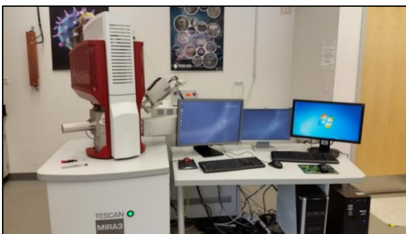
Figure 6. Scanning Electron Microscope (SEM) (TESCAN MIRA3 model) field emission instrument
