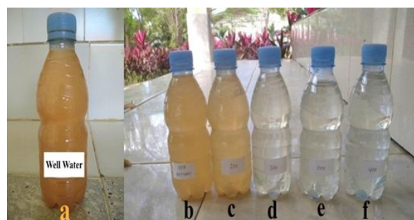
Figure 3. Initial samples of well water (a), water filtrated using sand without activation (b), water filtration results using microwave-activated sand with temperatures 250°C (c), 300°C (d), 350°C (e), and 400°C (f)
