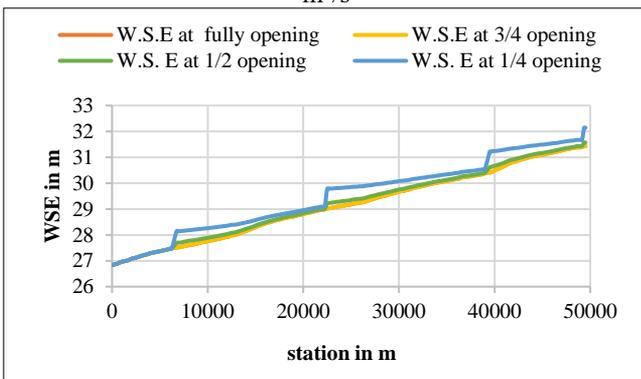
(c) WSE in m, when flow rate ranged between 30 to 35 m<sup>3</sup>/s
