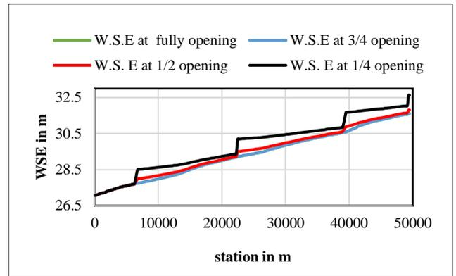
(e) WSE in m, when flow rate ranged between 35 to 40 m<sup>3</sup>/s
