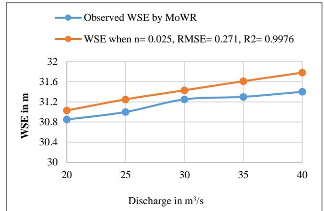
Figure 8. Validation of unsteady-state flow model in the reach of study for the period from February to June 2021 at Musayyab Head Regulator
