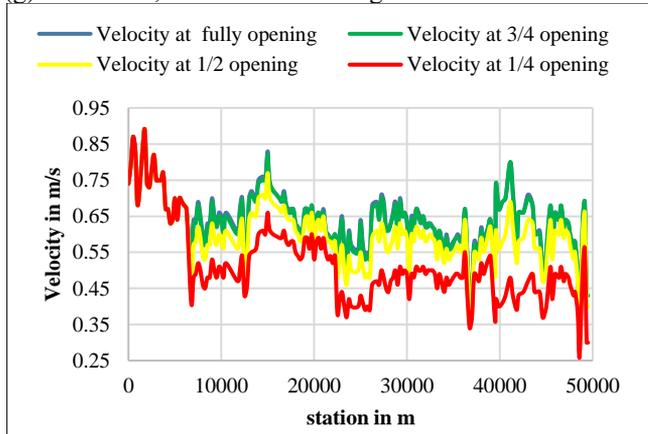
(h) Velocity in m, when flow rate ranged between 40 to 45 m<sup>3</sup>/s
