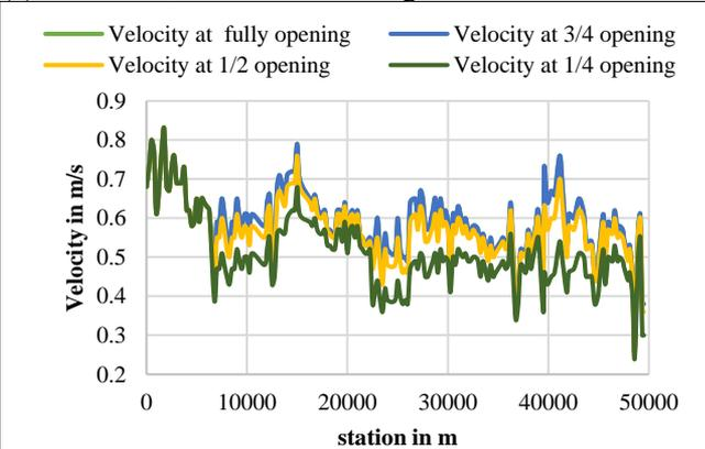
(d) Velocity in m, when flow rate ranged between 30 to 35 m<sup>3</sup>/s
