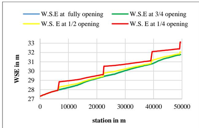
(g) WSE in m, when flow rate ranged between 40 to 45 m<sup>3</sup>/s
