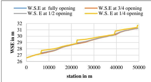
(a) WSE in m, when flow rate ranged between 25 to 30 m<sup>3</sup>/s
