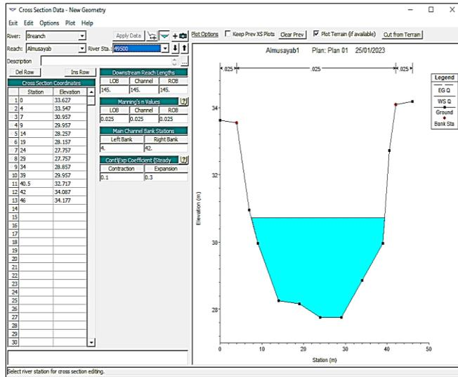
Figure 4. The cross-section geometrical data upstream cross-section
