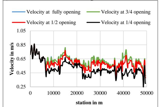
(f) Velocity in m, when flowrate ranged between 35 to 40 m<sup>3</sup>/s
