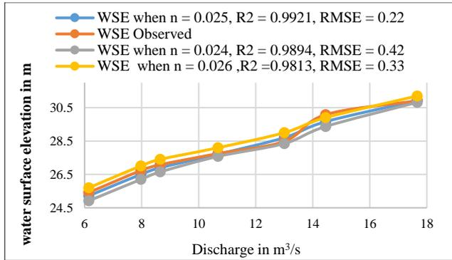
Figure 5. Calibration of steady-state flow model by the observed data
