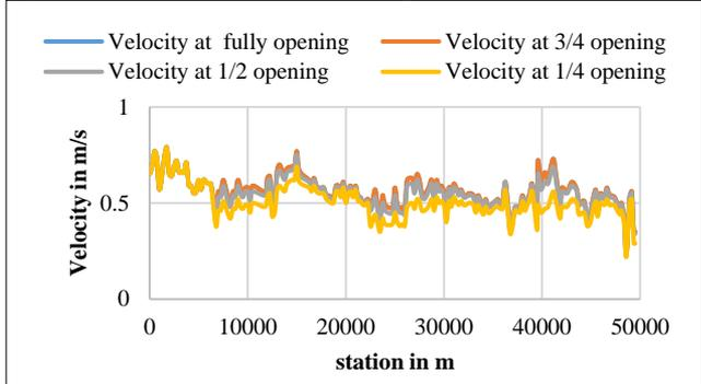
(b) Velocity in m, when flow rate ranged between 25 to 30 m<sup>3</sup>/s
