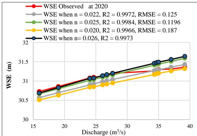
Figure 6. Calibration of unsteady-state flow model in 2020
