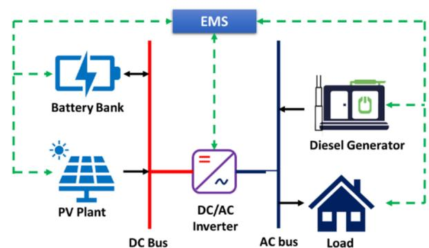
**Figure 1.** The model HES subjected to sizing optimization
