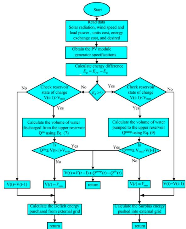
**Figure 3.** Flowchart describing the operation of HES
