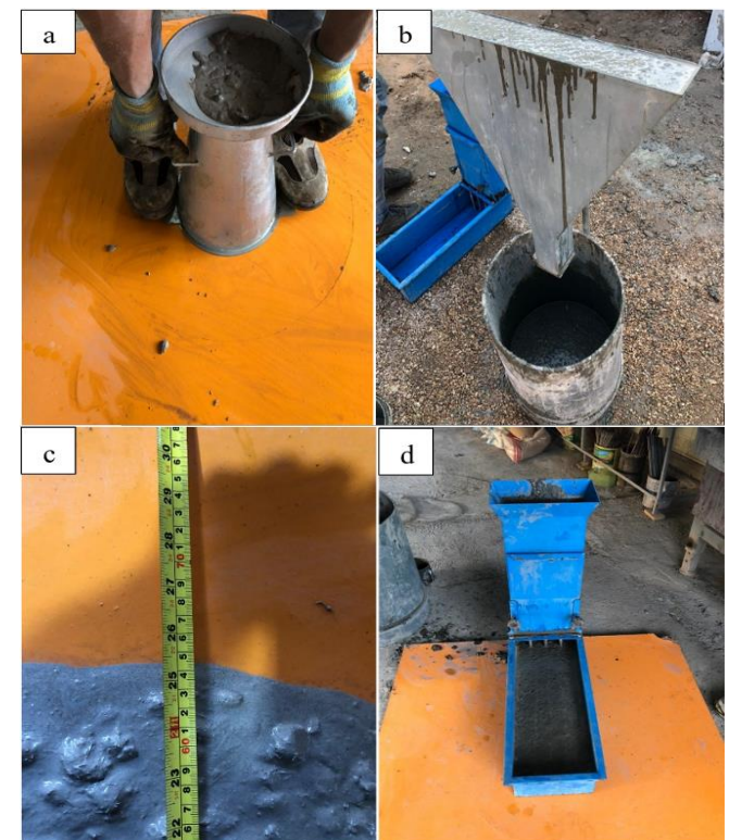
Figure 2. (a) D slump flow; (b) V-Funnel; (c) T50 flow; (d) L-box
