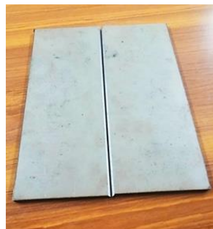
Figure 1. Welding test plate configuration
