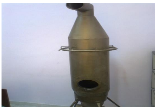
Figure 1. Cooling tower model
