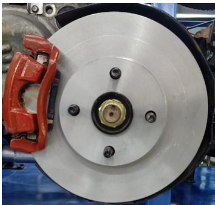
Figure 1. Disk brake assembly with a rotor and a caliper
