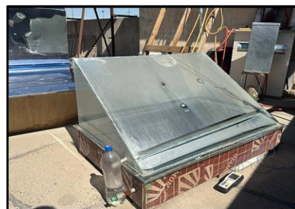
Figure 1. Photo of conventional solar still
