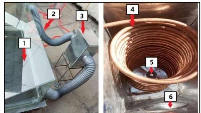
(1) glass of solar still, (2) hose of vapor, (3) the condenser, (4) heat exchanger, (5) distilled water collection hole, (6) the vapor inlet
