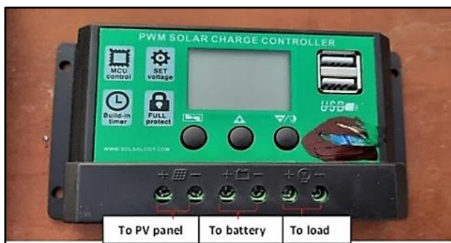
Figure 8. Solar charge controller device
