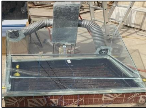
Figure 2. Photo of modified solar still
