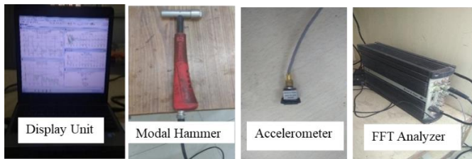
Figure 5. Modal testing arrangement set-up
