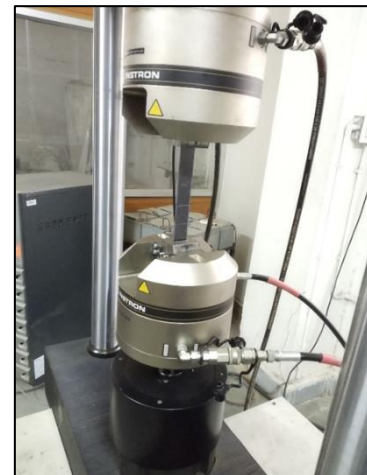
Figure 4. Tensile testing using INSTRON 8862
