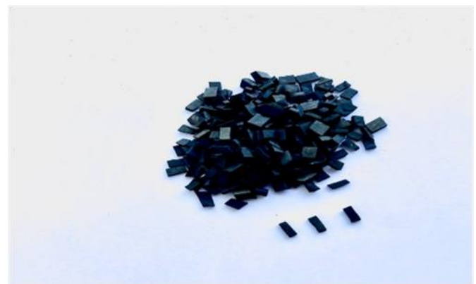
Figure 1. RW granules shredded from tire
