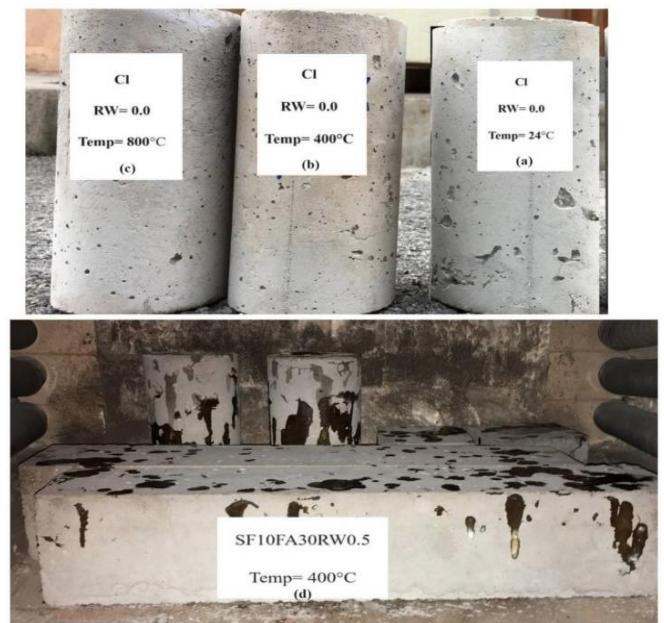
Figure 5. Effect of various temperatures on specimens surface
