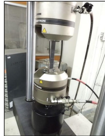
Figure 4. Tensile testing using INSTRON 8862
