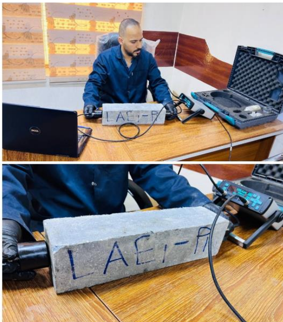
Figure 15. The test of UPV for A-EPSC specimens
