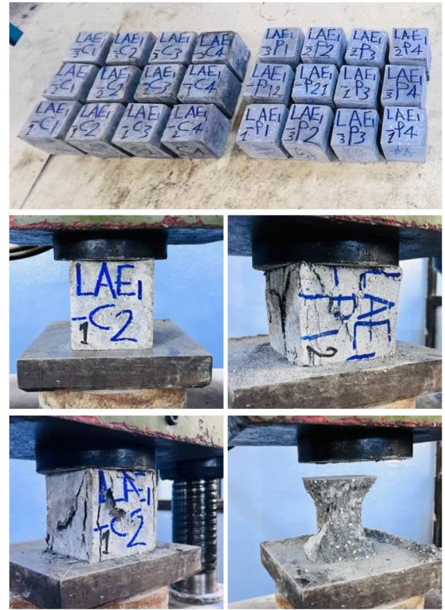
Figure 8. Compressive strength test for A-EPSC specimens
