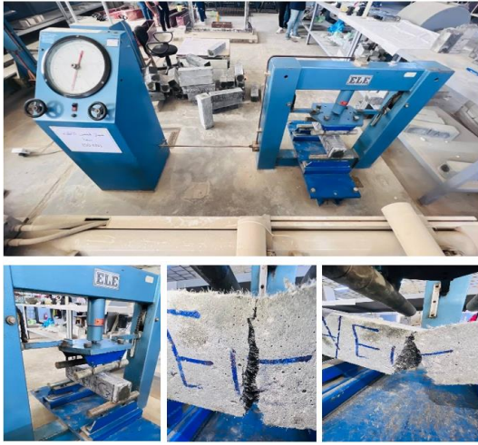
Figure 10. Flexural strength test and failure for A-EPSC specimens
