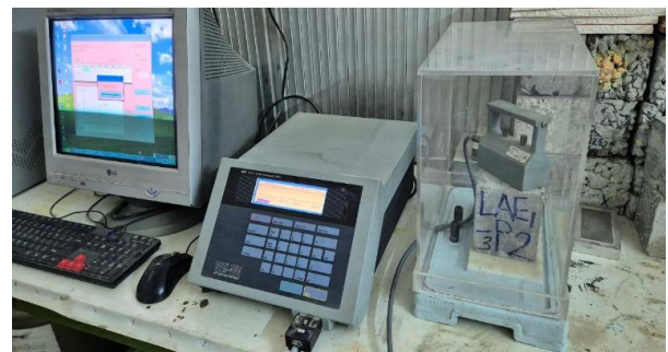
Figure 17. Thermal conductivity test of A-EPSC specimens
