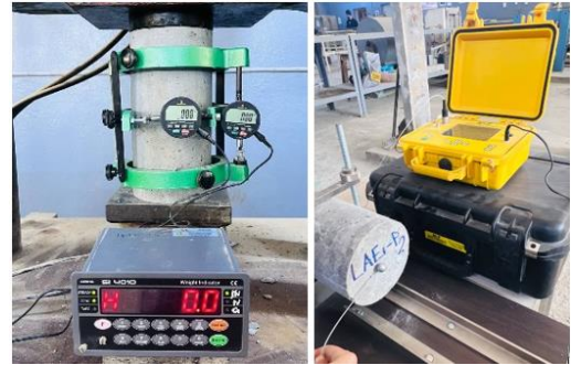
Figure 12. Static and dynamic modulus of elasticity tests
