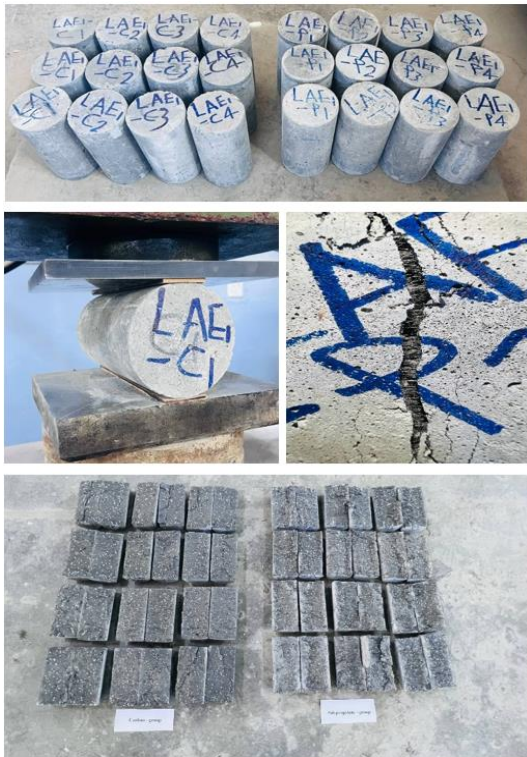
Figure 11. Splitting tensile strength test for A-EPSC specimens
