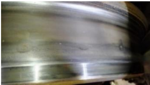
Figure 8. A wheel flat developed at the center of the contact area due to blockage or partial blockage on the seventh wheelset of metro train ID-108
