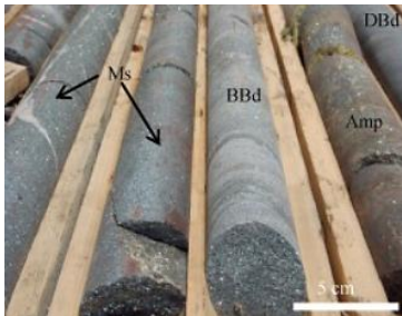
Figure 2. Drill holes with massive texture, bands of chalcopyrite and amphibolite
