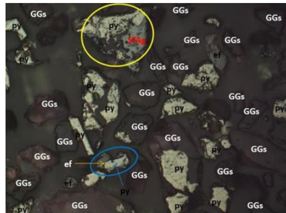
Figure 15. Mixed particle of silver sulfosalts and pyrite (SFAg/py) in yellow circle and mixed particle of sphalerite and pyrite (ef/py) in the blue circle
