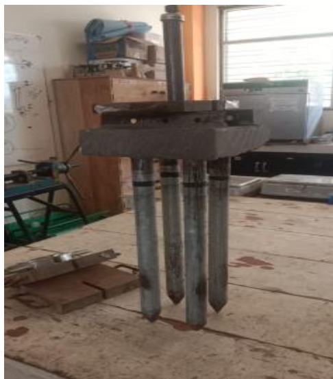
Figure 10. 2×2 group pile foundation model
