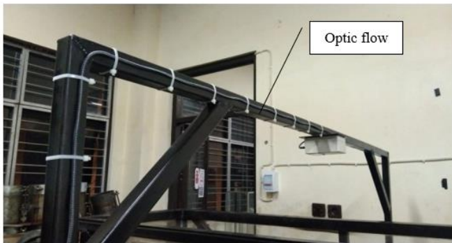
Figure 5. Placement of optic flow sensor on rigid container
