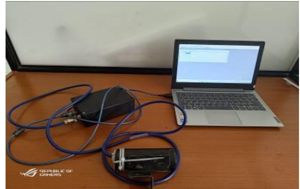
Figure 4. Soil pore water pressure test equipment
