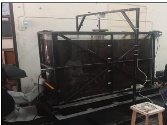
Figure 3. Photo of shaking table and rigid container equipment
