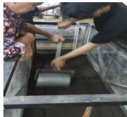
Figure 9. Compaction trial on rigid box
