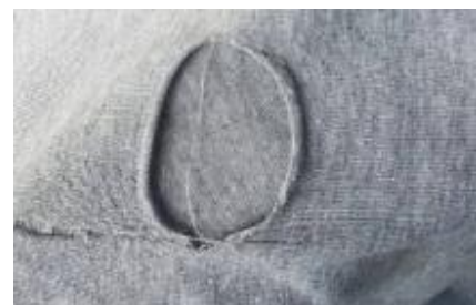
Figure 2. Knitted fabric with loose threads
