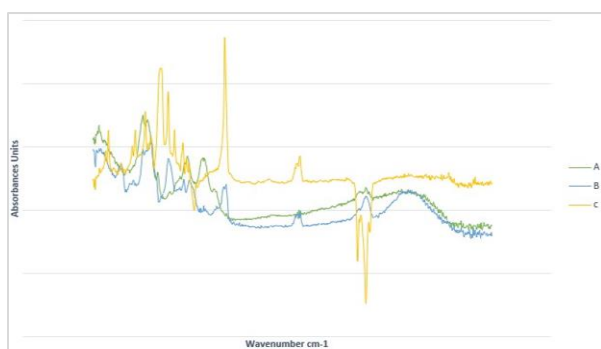
Figure 1. Fourier Transform Infrared Spectroscopy (FTIR) Analysis A) cs; B) PVA; C) PVA+cs
