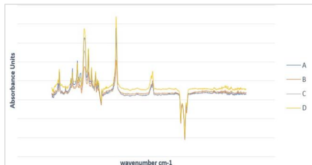
Figure 3. Fourier Transform Infrared Spectroscopy (FTIR) Analysis: A) PVA+CS; B) PVA+CS/0.02TiO 2 ; C) PVA+CS/0.04TiO 2 ; D) PVA+CS/0.06TiO 2
