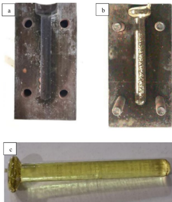
Figure 2. Casting of glass sample for dilatometer test: (a) and (b): The mold two sides; (c) Glass cast for dilatometer
