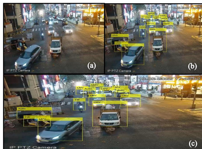
Figure 8. (a) Sample input video-frame; (b) object detection using Yolo-v2 and (c) vehicle type classification from LSTM-OWHO for Night-time condition
