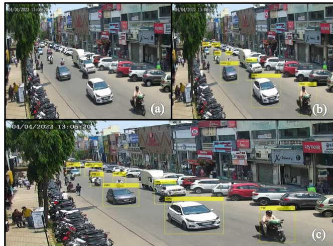
Figure 6. (a) Sample input video-frame; (b) object detection using Yolo-v2 and (c) vehicle type classification from LSTM-OWHO for day-time condition
