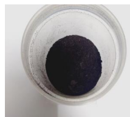
Figure 5. Sample of synthesized by a burst of light flash graphene
