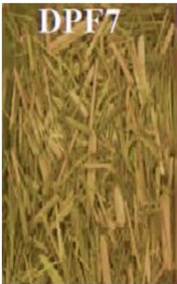
**Figure 1.** Date palm fiber with a length equal to 7 mm (DPF7)
