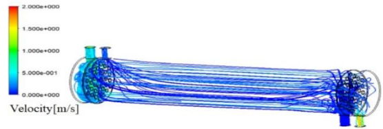
Figure 17. Streamline velocity distribution of the STHE
