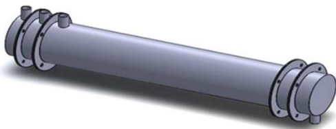
Figure 4. Representation of the CWST heat exchanger
