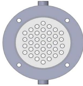
Figure 3. Representation of the tube arrangement inside the STHE
