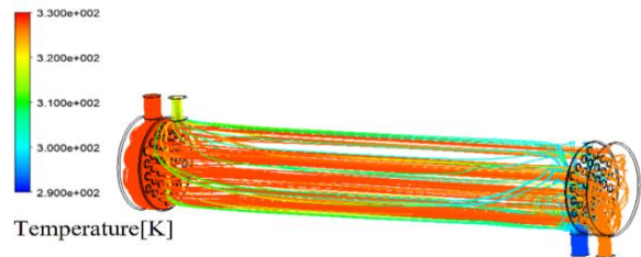
Figure 21. Streamline temperature distribution of the STHE
