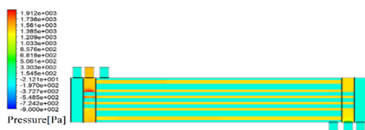
Figure 10. Longitudinal section figure that represents pressure distribution of the CWST heat exchanger
