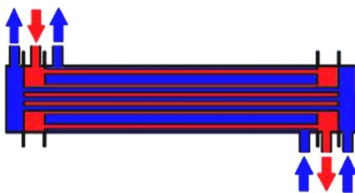
Figure 8. Representation of the hot (red) and cold (blue) fluids in longitudinal section of the CWST exchanger
