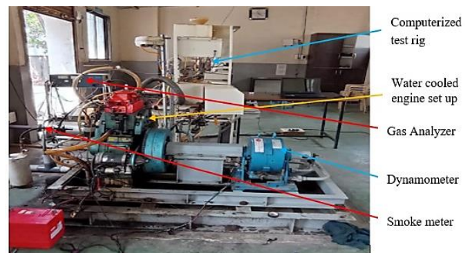
Figure 1. Engine test bed
