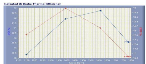
Figure 6. Variation of Indicated, and brake thermal efficiency speed
