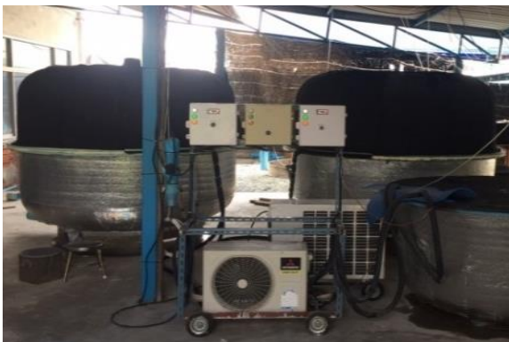
Figure 10. Temperature and oxygen control system prototype
