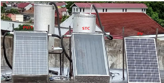
Figure 1. PV/T, STC, and PV systems
