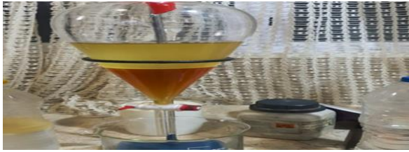
Figure 2. The process of separating biodiesel from glycerin after stratification process
