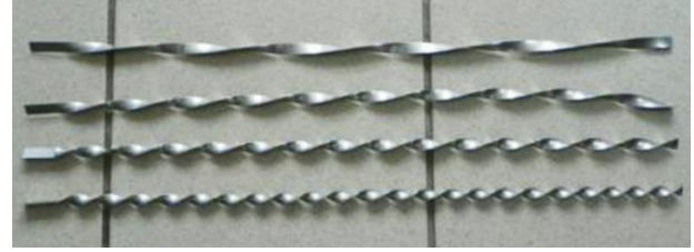
Figure 2. Strip turbulizers used by Wiśniewska [26]
