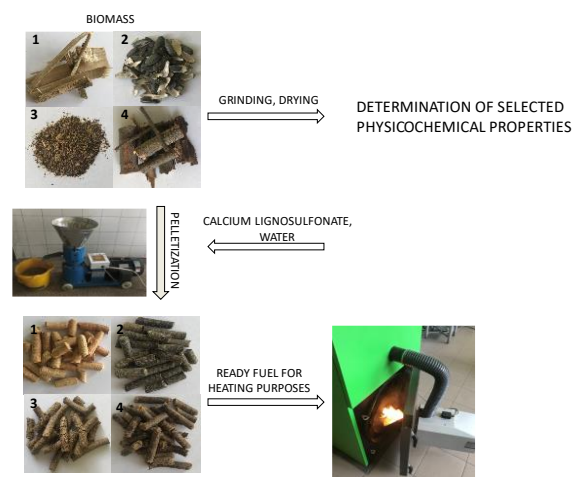
Figure 1. Schematic diagram of preparation of selected types of biomass for heating fuel, where: 1 - pine, 2 - sunflower husk, 3 - rapeseed cake, 4 - willow ( Salix viminalis )
