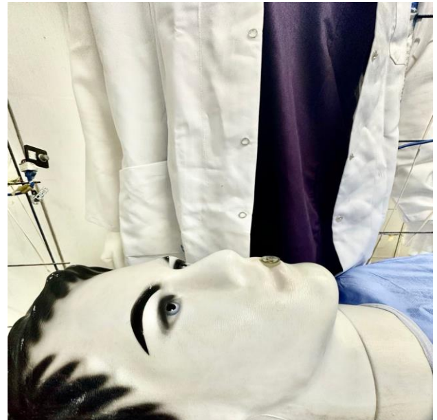
Figure 2. Thermal breathing manikins were used in this study to simulate the patient
