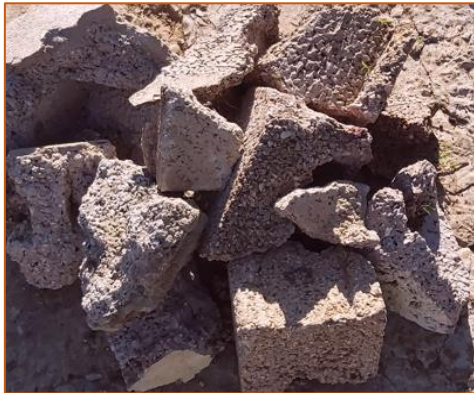
Figure 1. Hollow concrete blocks waste
