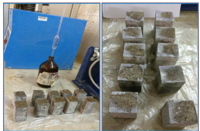
Figure 7. Measuring chloride penetration depth
