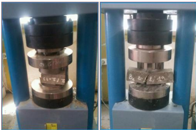
Figure 6. Compression and flexural tensile strength test
