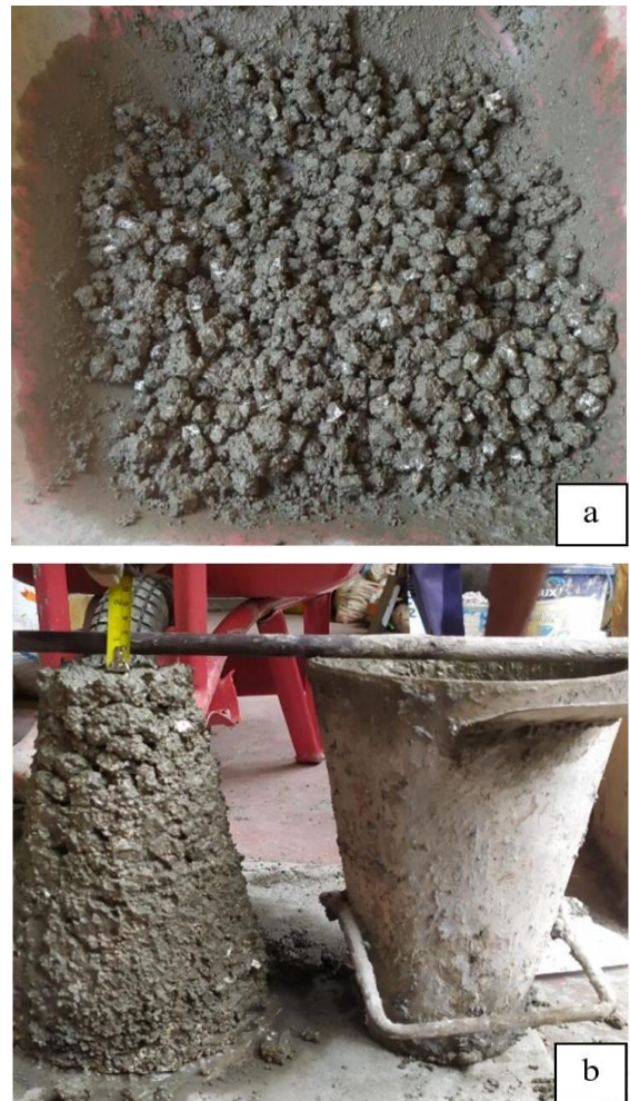
Figure 6. a) fresh lightweight concrete mix b) slump value
