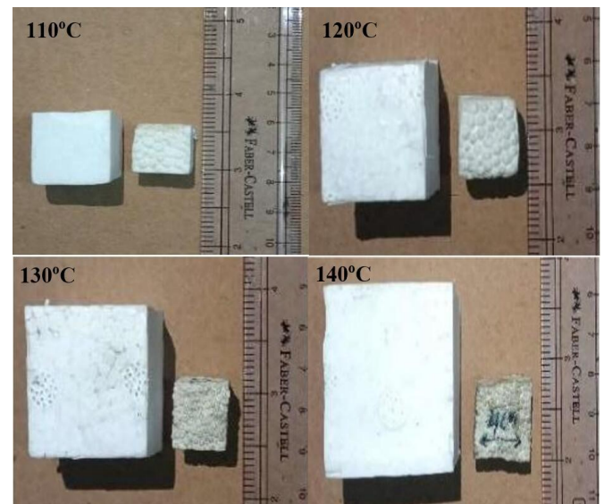
Figure 1. Volume change of EPS aggregate due to heating
