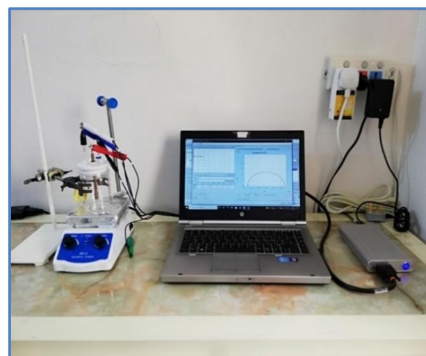
Figure 2. The system of corrosion/EIS measurement
