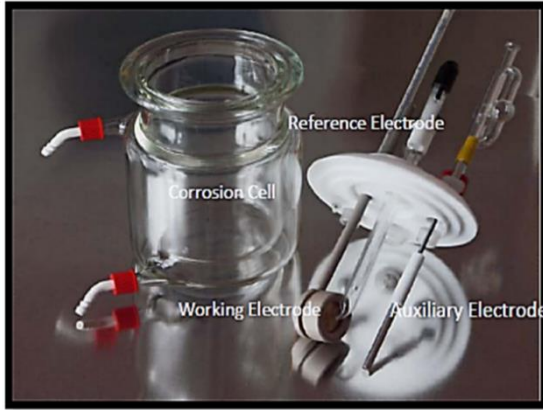
Figure 3. Set up the corrosion cell and three electrodes
