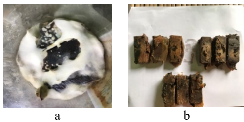
Figure 2. Teak wood samples before testing (a) and after testing (b) with P. sanguineus fungus
